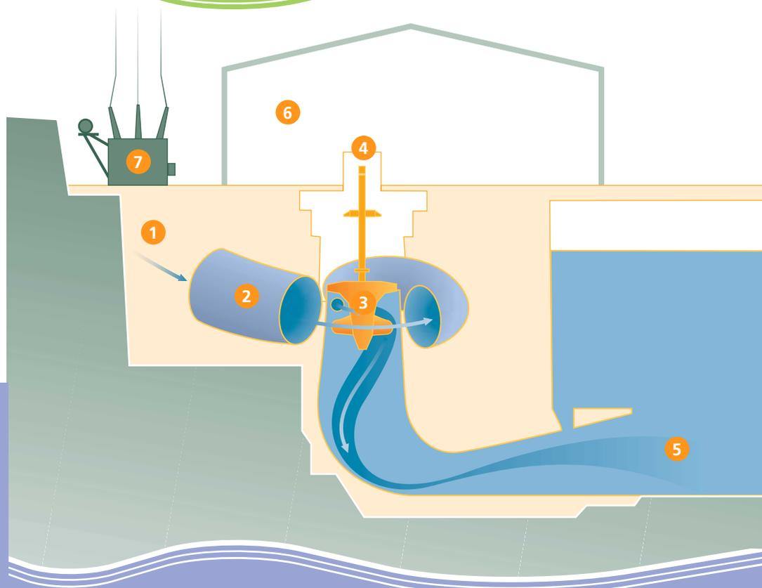
Dams are built across rivers to hold back the water. The water is then directed through big pipes (penstock) and falls against the blades of giant turbines.
